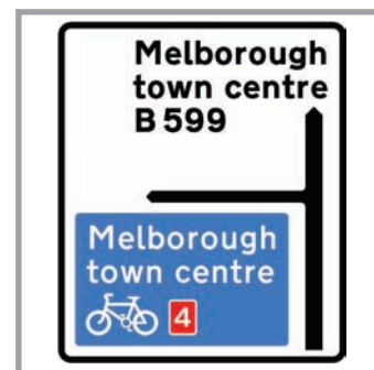
Advanced direction sign on the highway approach to a National Cycle Network route, Diag. 2105.1 (1)
